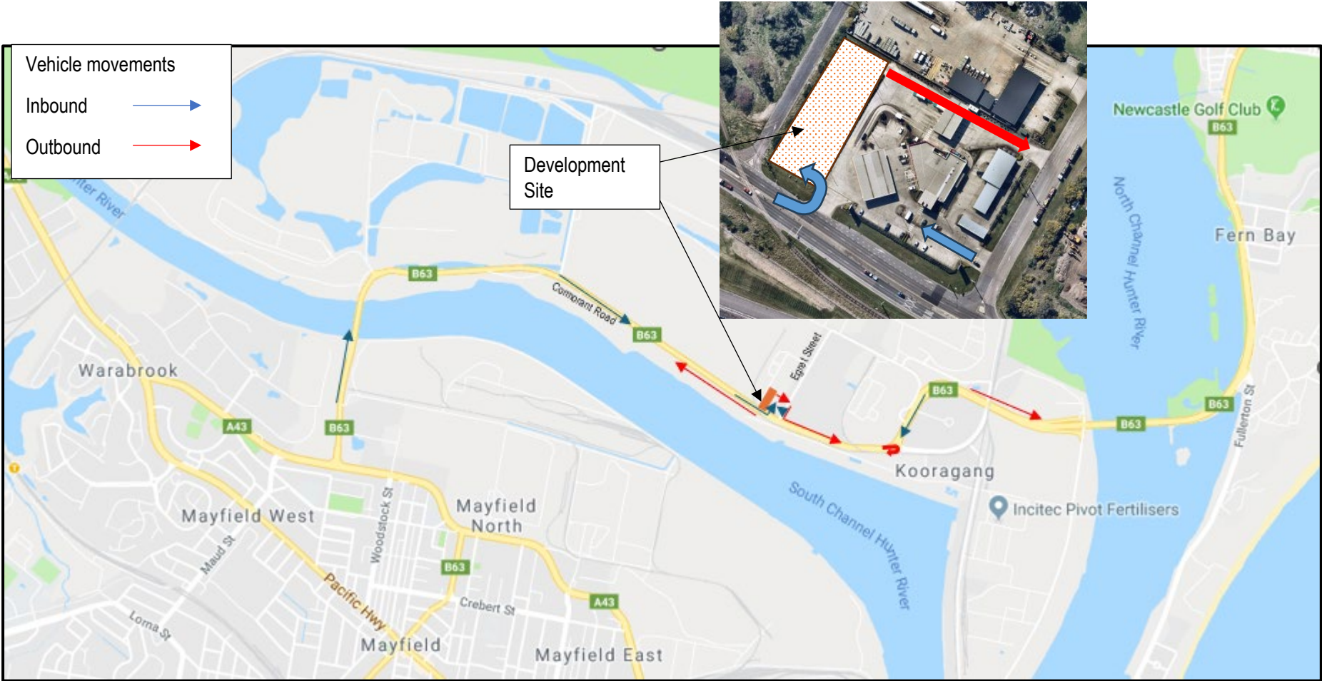
Figure 1 Vehicle Movement Plan within context of broader road network demonstrating inbound and outbound demands
